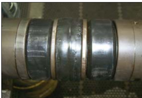
This bottom packer (left photo) was retrieved from Well 3 after an unsuccessful set; note position of elements and slips (Fig. 5). The elements of the lower packer (right photo) were retrieved from Well 3. It's clear that the middle element has been extruded, but not as obvious that the outer two elements have been extruded (Fig. 6).
