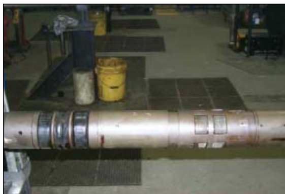
This bottom packer (left photo) was retrieved from Well 3 after an unsuccessful set; note position of elements and slips (Fig. 5). The elements of the lower packer (right photo) were retrieved from Well 3. It's clear that the middle element has been extruded, but not as obvious that the outer two elements have been extruded (Fig. 6).
